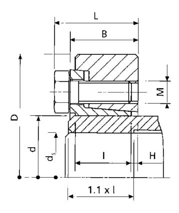
B mm = 38.0d H8 mm = 90D mm = 155.0ds mm = 65F kN torque = 185
